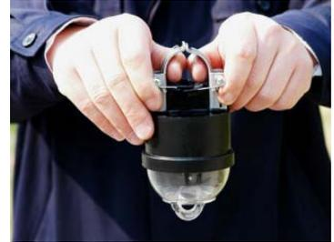
2) Once the Split Coil CT has been cocked, the line holding springs will automatically engage, locking the unit in the "open" position.
