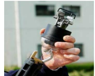
4) Position the conductor between the open Split Coil CT, and with a forceful upward movement, install the device to the line. When the Spring Release Trigger receives sufficient pressure, the spring will release clamping the conductor and setting the device into place.
